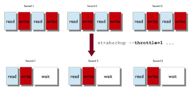
By default, there is no throttling, and **xtrabackup** reads and writes data as quickly as it can. If you set too strict of a limit on the I/O operations, the backup might be so slow that it will never catch up with the transaction logs that InnoDB is writing, so the backup might never complete.
